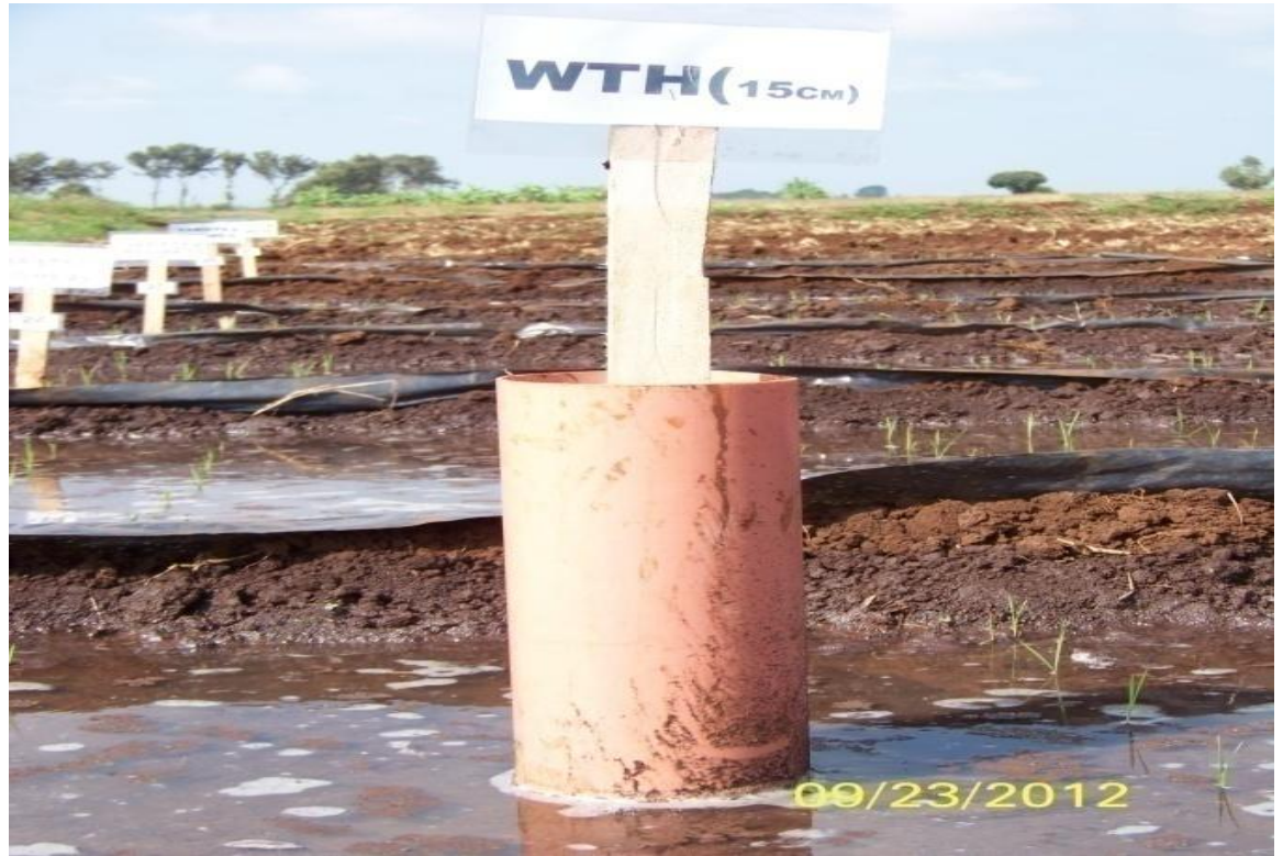
Figure 7: Water threshold level gauge (15 cm below soil surface)
