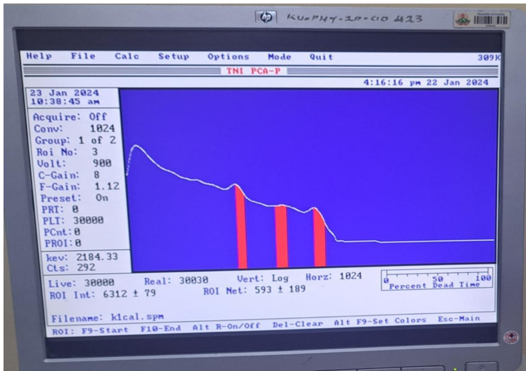
Figure 7: A screenshot of regions of interest in the spectrum taken for one of the samples
