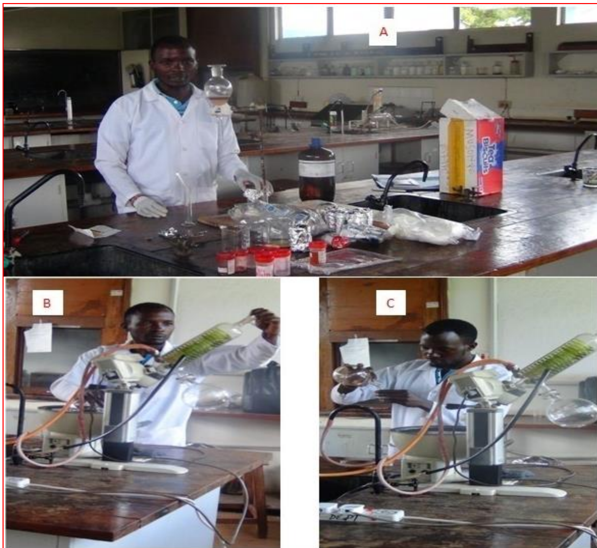
Plate 3.3: Urine extraction and clean up steps showing; A- LLE by use of DCM, B- Concentrating the sample at 40^{\circ}\text{C} on a rotary pump and C-Dispensing the final extract product in a bijou bottle.
