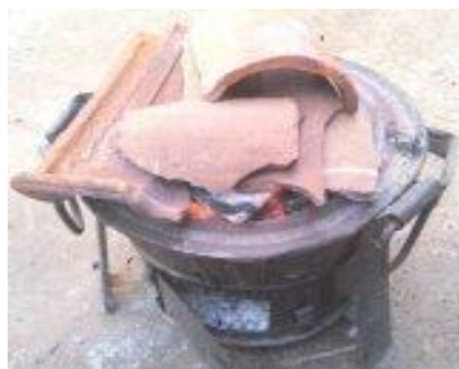
Plate 3.2 : Charcoal Jiko with laterite-charcoal mixture heated in a controlled air current.
