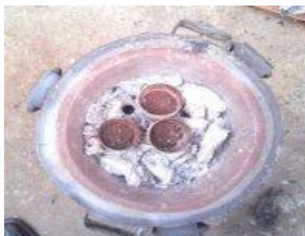
Plate 3.1 : Charcoal Jiko with fire clay crucibles containing laterite-charcoal mixture.
