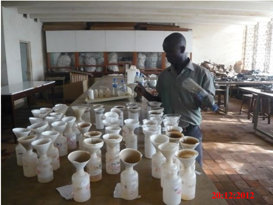
Plate 3.5: Sediment filtration for soil and nutrient loss determination
