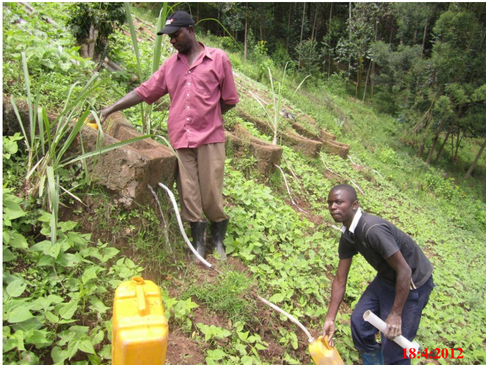
Plate 3.3: Calibration of the runoff plots
