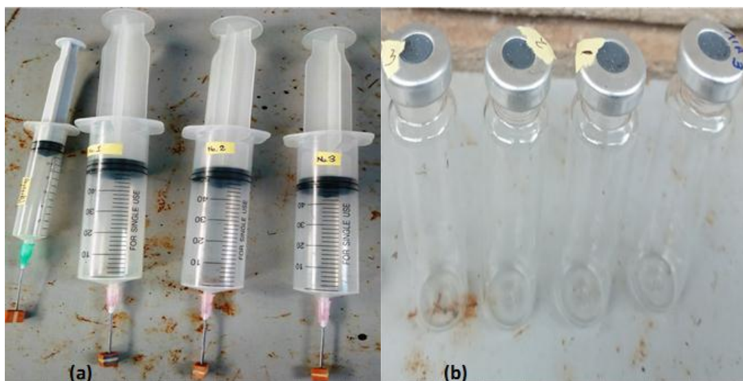
Figure 3.5 (a). Producer gas and air samples for analysis at JKUAT, (b). Producer gas and air samples for analysis at ILRI
