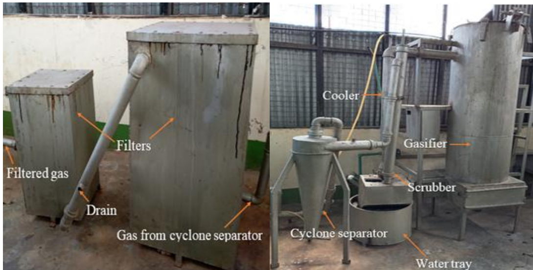
Figure 3.4 Schematic diagram of gasification plant at JKUAT.
