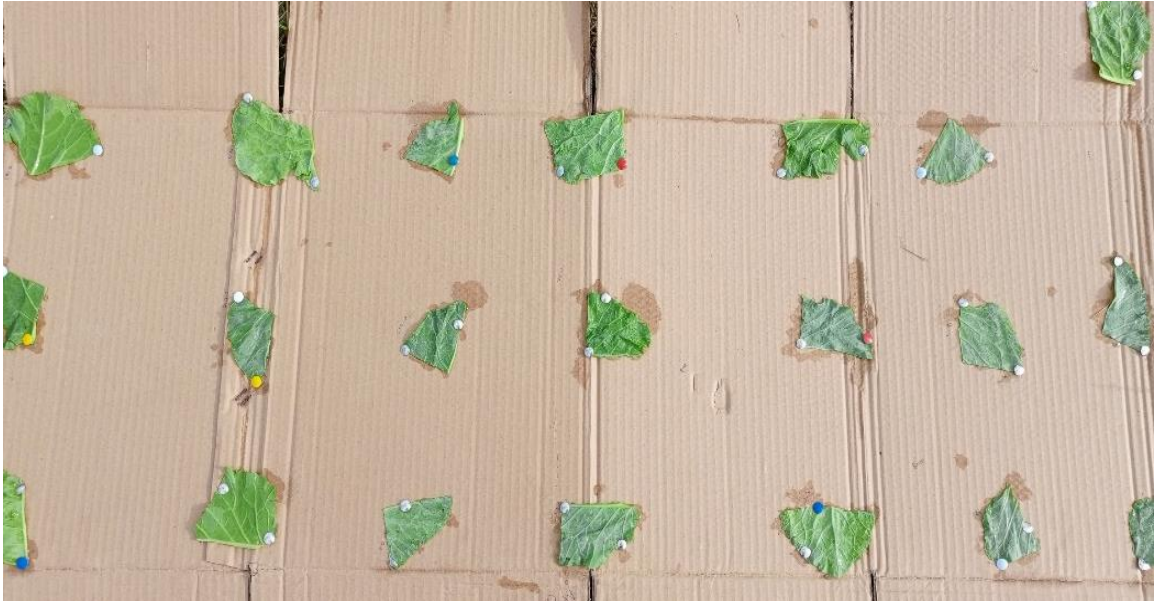
Figure 3.2: Kale samples containing different concentrations of chlorpyrifos. Spacing between the samples was carefully chosen to prevent the different chlorpyrifos concentrations applied from interfering with one another.
