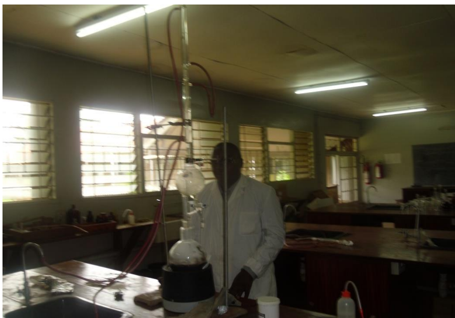
Figure 3.1: Extraction of N. sativa seeds essential oil using hydro-distillation apparatus
