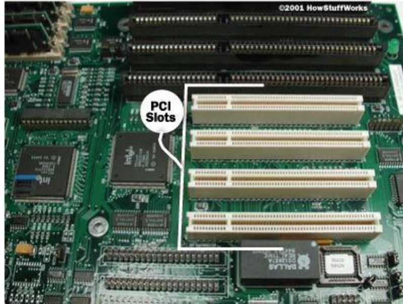
Fig. 3.10: A photograph of PCI slots on a computer motherboard (Intel, 1995).
