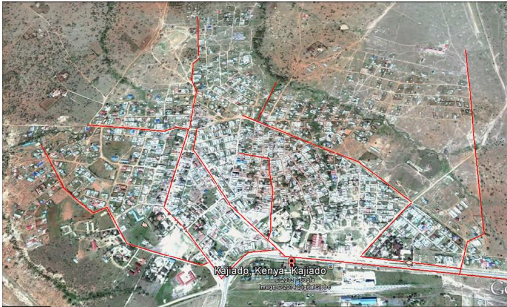
Figure 5.11: Map of Kajiado town showing the proposed water distribution system. Modified from Google maps.
