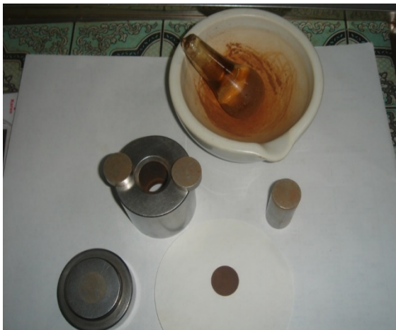
Plate 3.19: pellet dice, mortar and pestle
