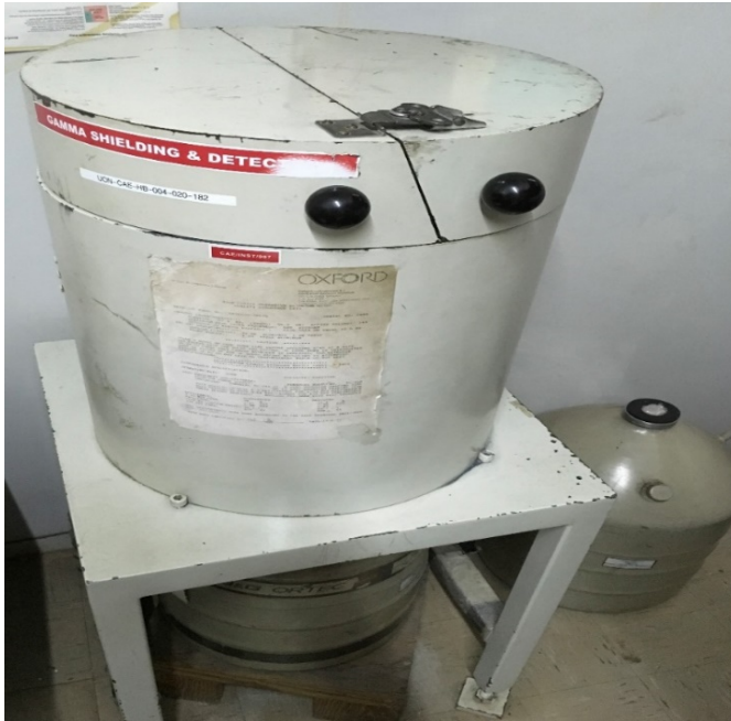
Plate 3.16: HPGe detector at the INST-University of Nairobi.
