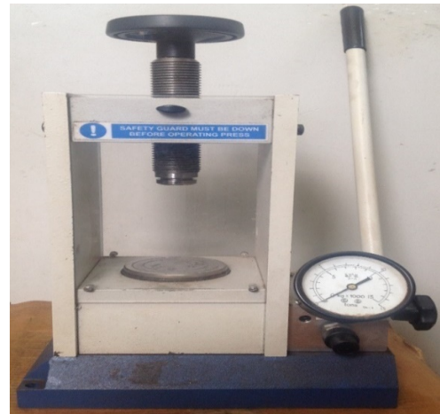
Plate 3.18: Hydraulic press machine
