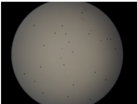
Figure 3.9: Typical image of formed tracks in the CR-39.
