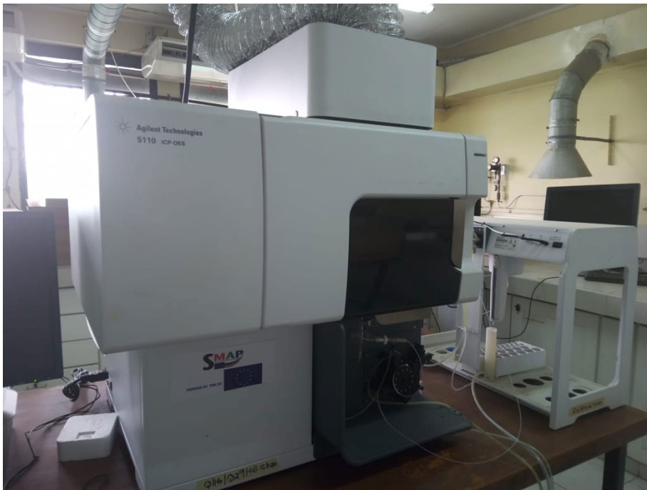
Plate 3.21: The ICP-OES at Kenya Bureau of Standards
