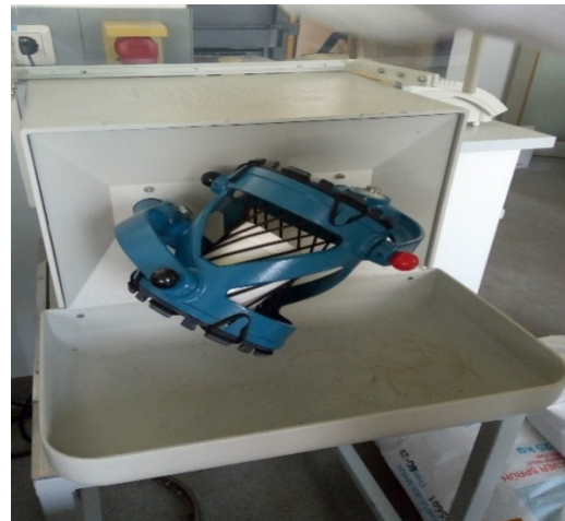
Plate 3.13: Soil sample mixer
