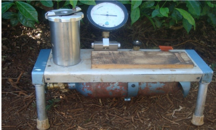
Plate 3.3: Pressure chamber: Measuring the xylem water potential of tea shoots (Model 1515D)
