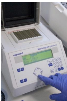
Figure 3.6: A Thermo-cycler used in PCR reaction
