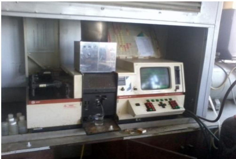
Plate 2.17 Atomic absorption spectrometer, model: varian spectr AA 10 (2005).
