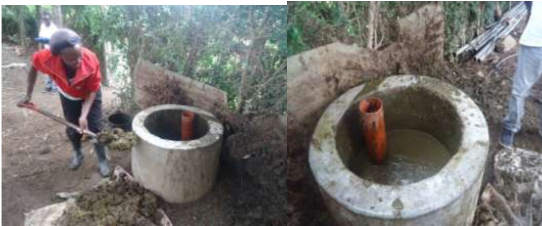
PLATE 7 (a) An adopter feeds the dung into the biodigester mixing trough (b)The mixture of the cow dung and water ready to be released into the digester
