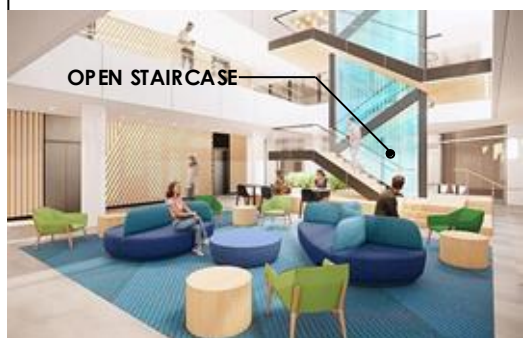
Figure Atrium. Source: https://capitalprojects.mit.edu/projects/w20 Introduction of a three-story atrium allows natural lighting of the building. Use of open staircases and glass railings around the atrium to allow light travel.
