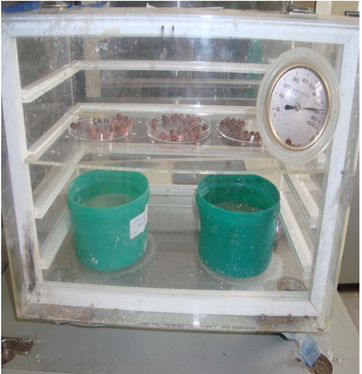
Figure 3.2: Desiccant Samples under Sorption Investigation in a Humidity Chamber
