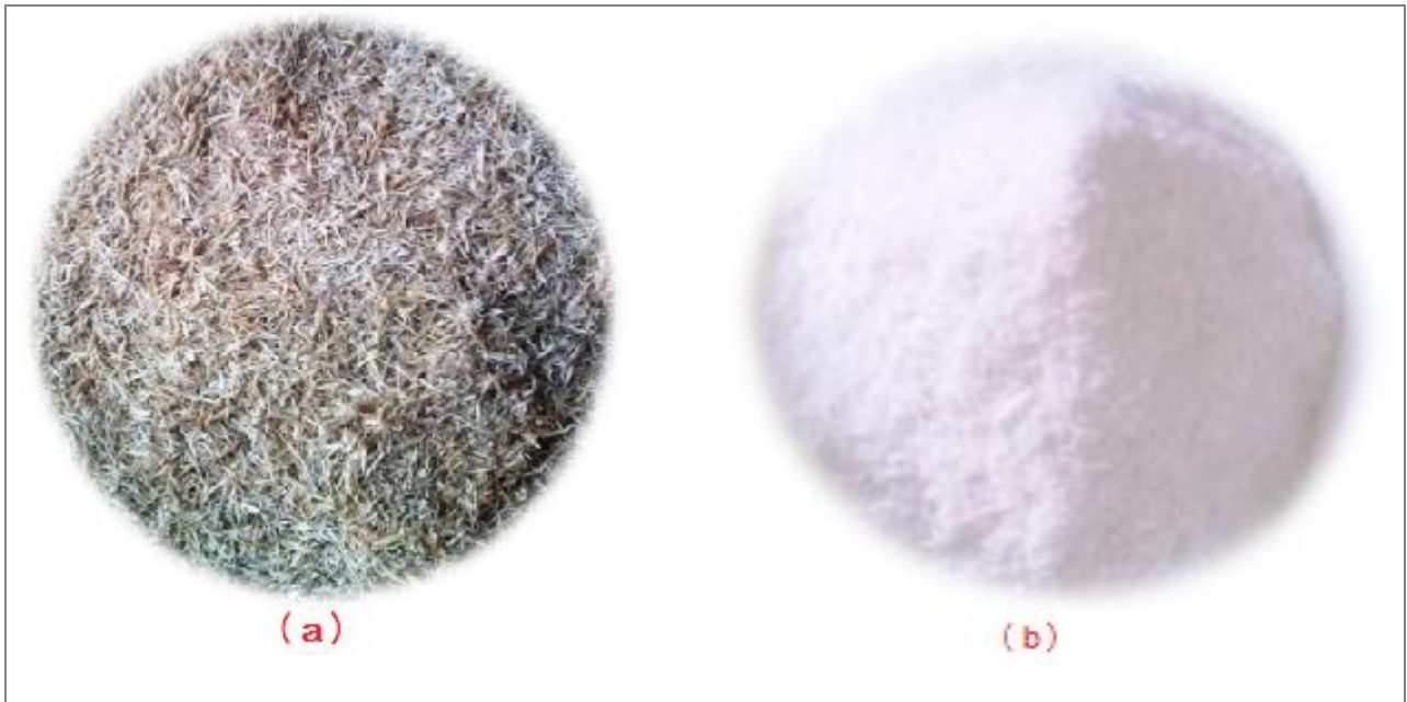
Figure 4.2: Carbonised Rice Husks (a); Completely Incinerated Rice Husks (b).
