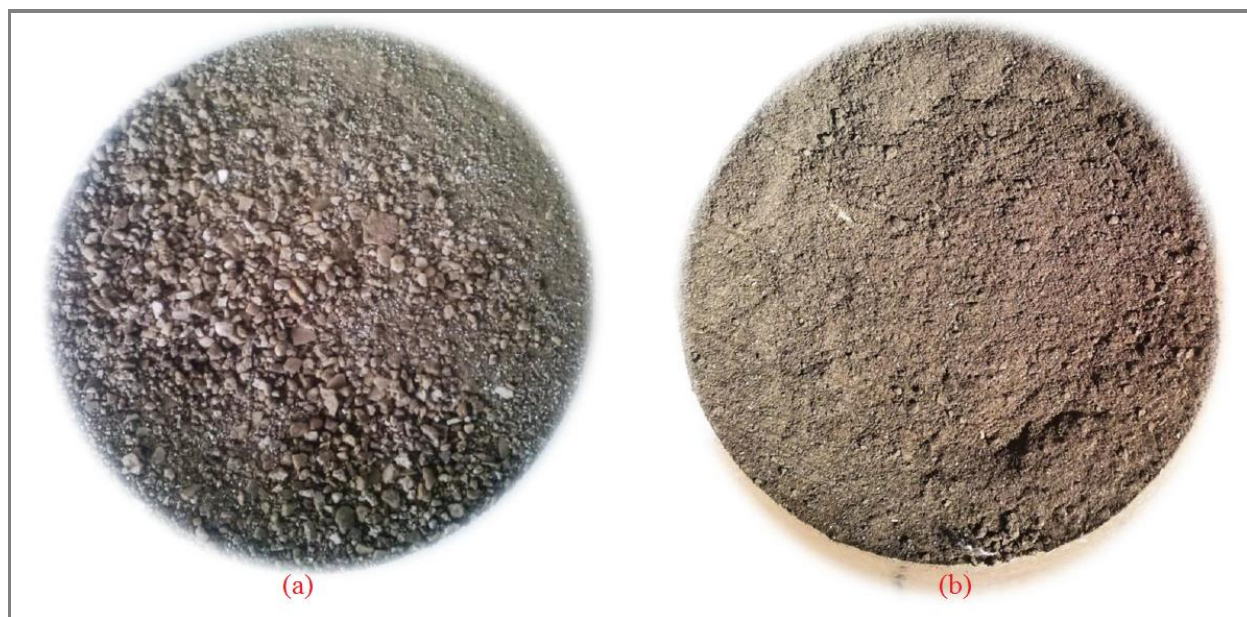
Figure 4.10: (a) Si/MgO mixture; (b) Synthesized Silicon nanoparticles.
