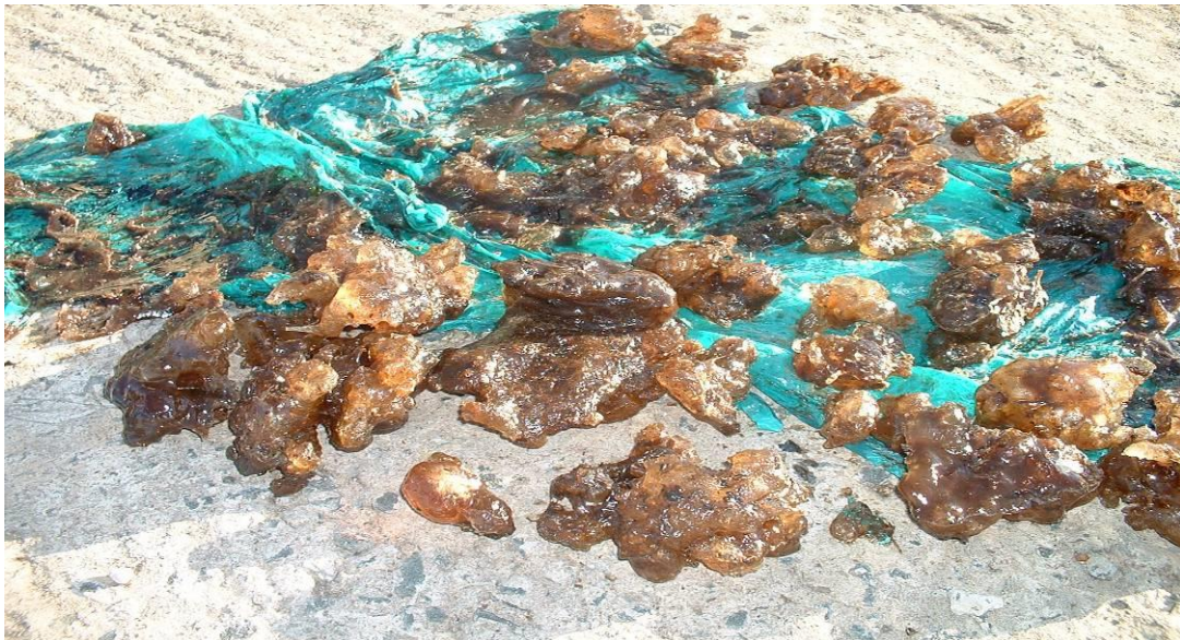
Fig 4.7: Gum Arabica used as a binder for making biomass fuel briquettes
