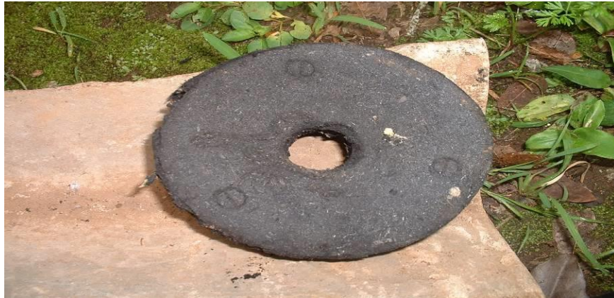
Fig 2.5: Carbonized bagasse briquettes
