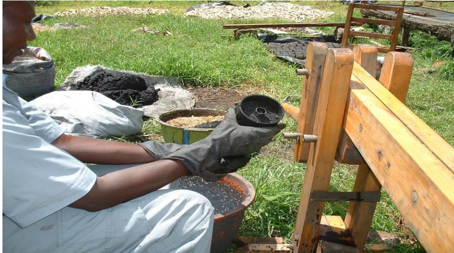
Fig 2.6: Fuel briquettes making from agro-based wastes, carbonized bagasse included
