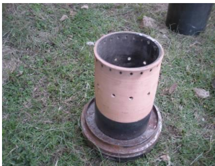
Fig 4.12: Stove liner fixed to the stove base
