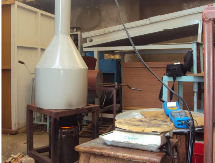
Figure 3.5: Photo showing emission testing of the semi-gasifier stove
