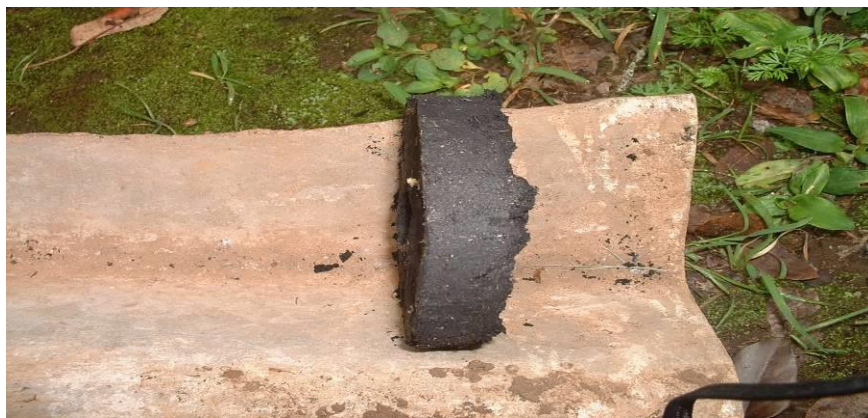
Fig 2.5: Carbonized bagasse briquettes
