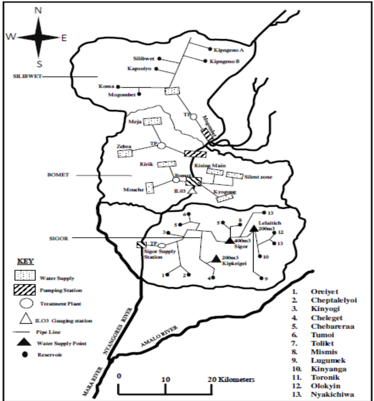
Figure 4.7: Piped water distribution network
