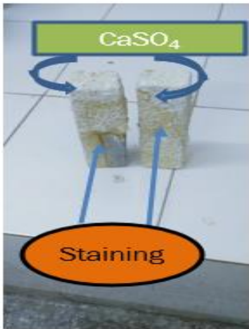
Plate 4.9: Mortar Prisms Exposed in sulphuric acid as a curing media
