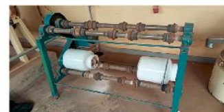
The porcelain grinding mill
