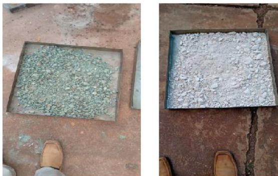
The crushed rocks using the ball mill
