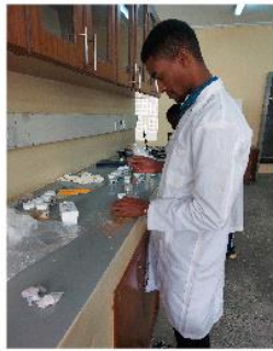
Putting the rock powder to the small tins for the chemical analysis.
