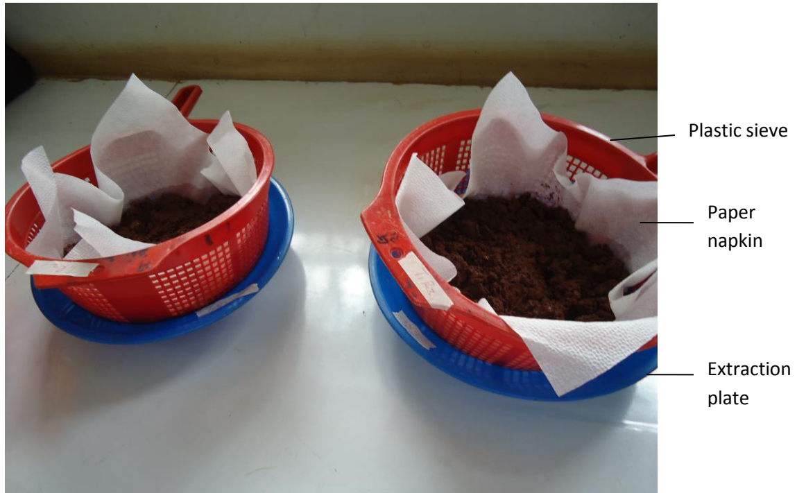
Plate 3.3: Extraction of J2s' from the soil using modified Baermann's method.
