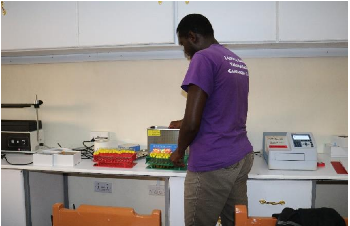
Plate 3. 12: Sonicating the extracts in an ultrasonic bath in the sonicator.
