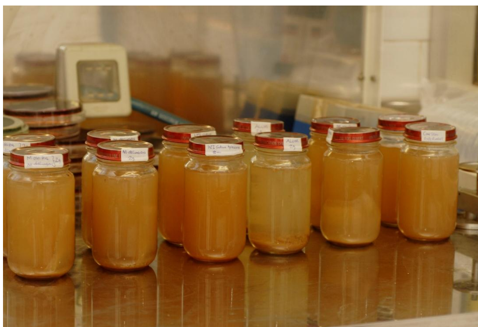
Figure 4 Setup showing incubation of water samples during treatment. Different samples show different turbidity levels
