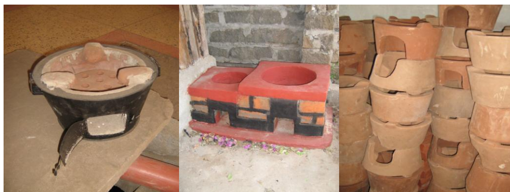
Plate 1: Improved modified Kuni Mbili stove, Rocket stove and Maendeleo liners made by SCODE
