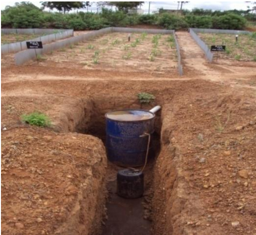
Plate 3.2: Runoff plot and collection tank (a) and an automatic rain gauge (b)
