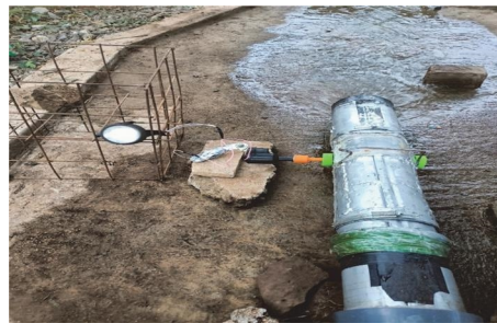
FIGURE 10: Demonstration of lighting by in-duct turbine at testing site in KUATC.
