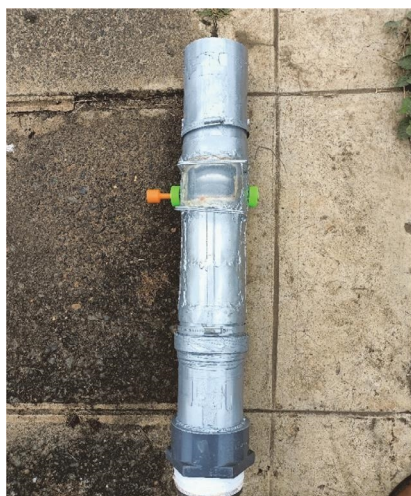
Plate 3.1: Fabricated turbine assembly
