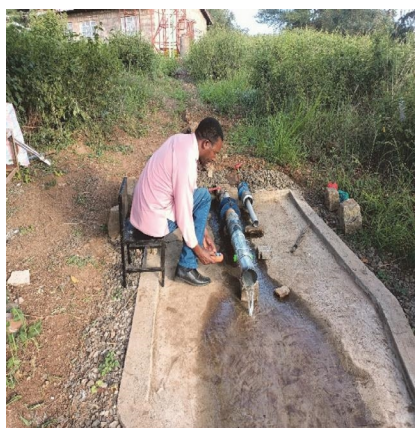
Plate 3.4: Reading RPM values using a tachometer
