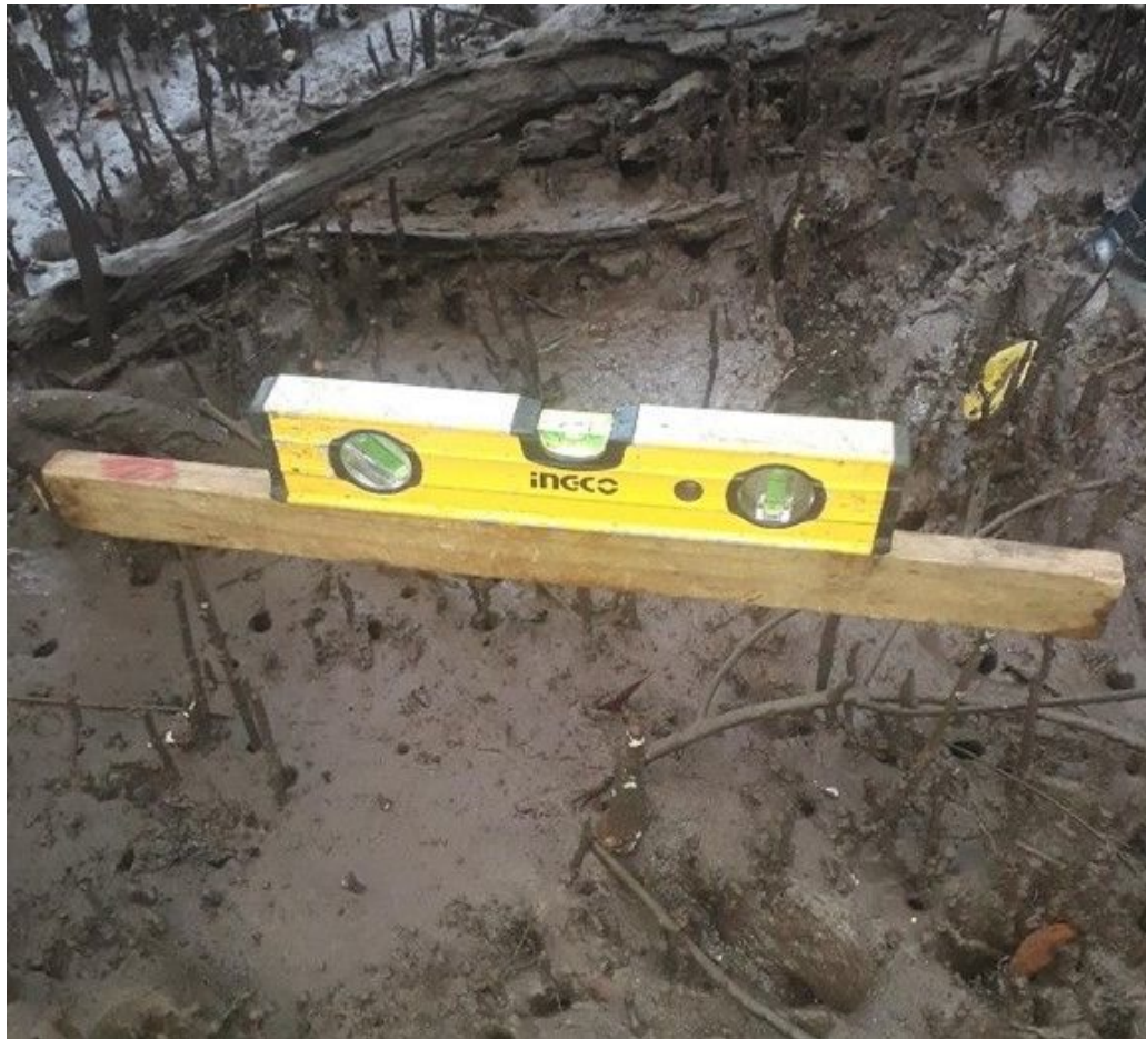
Plate 2: Sediment Elevation Tables (SET) installed to determine sediment elevation change.
