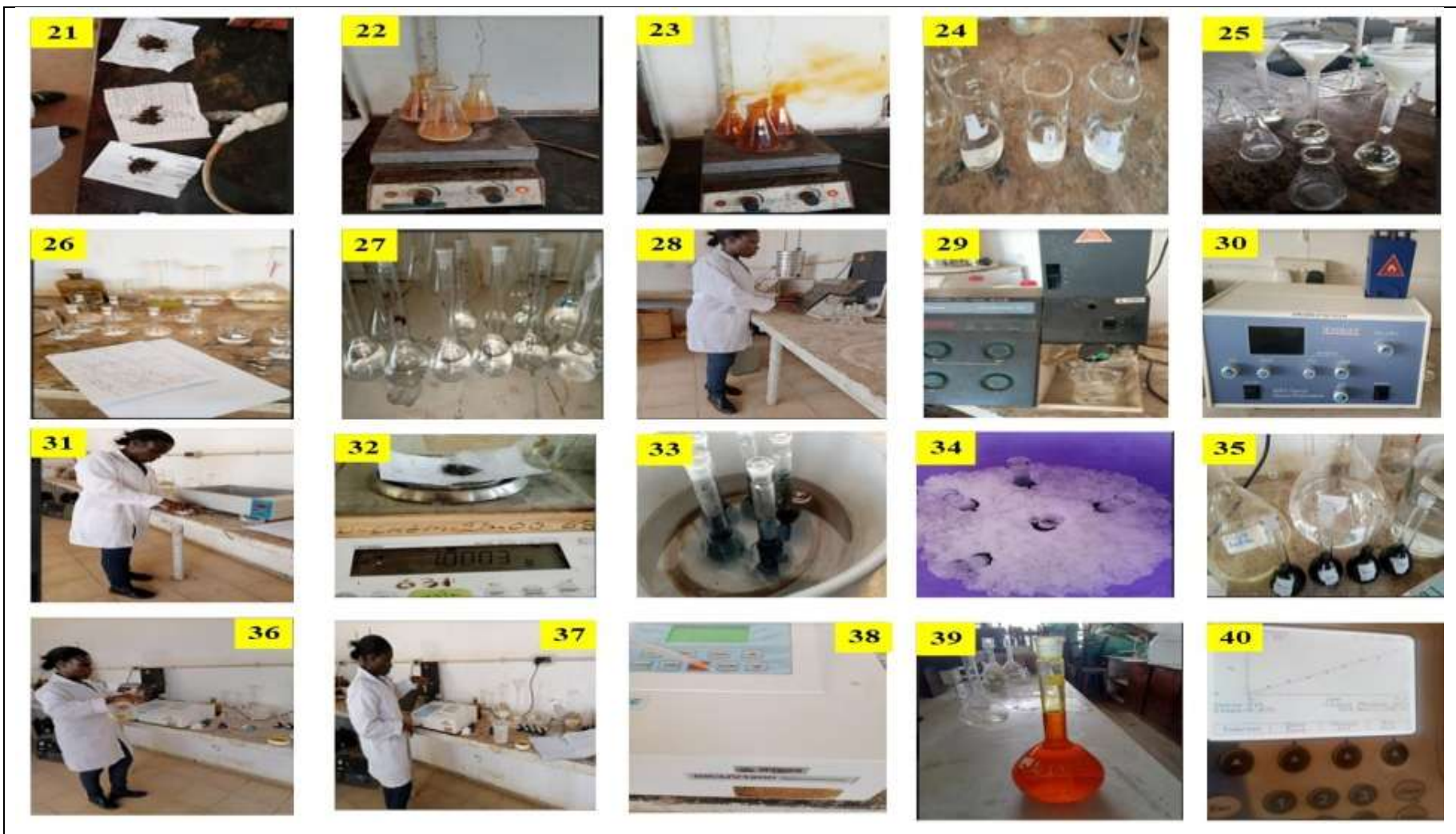
Figure 0-3: 21-30-Potassium and sodium determination using Flame Photometer. 31-38. Phosphorus and sulfur determination using U-V Spectrophotometer. 39. Potassium dichromate for Total Organic Carbon (TOC) determination and 40. Standard chart from U-V for TOC.
