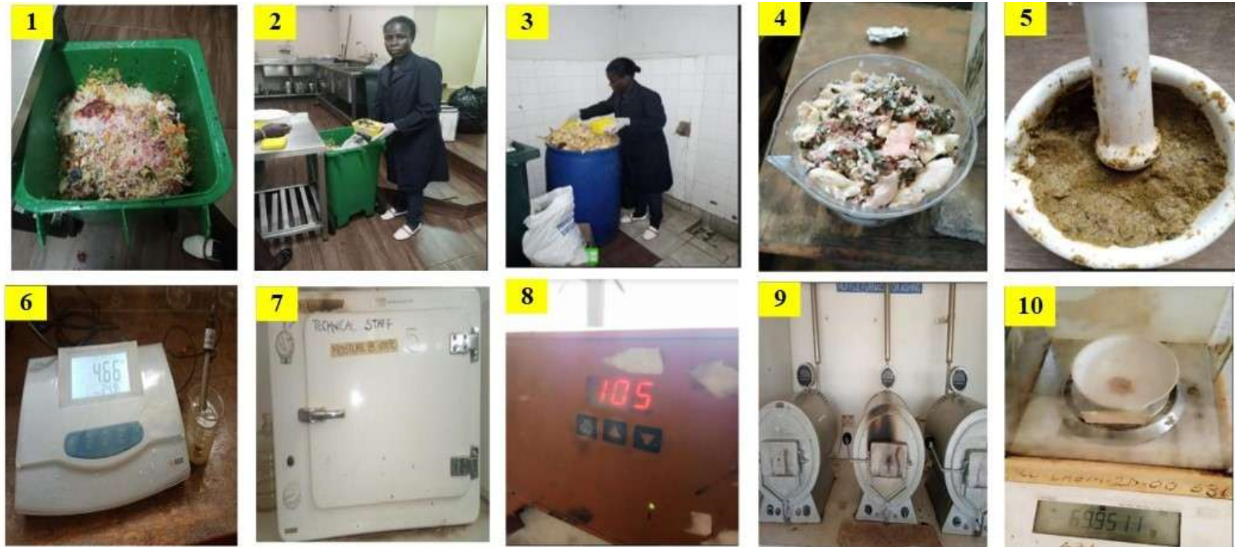
Figure 0-1: 1-4. Food waste collection & sampling, 5. Wet sample homogenized, 6. pH Measurement, 7-8. Oven @105 °C, 9. Muffle furnace 10. Ash weighing
