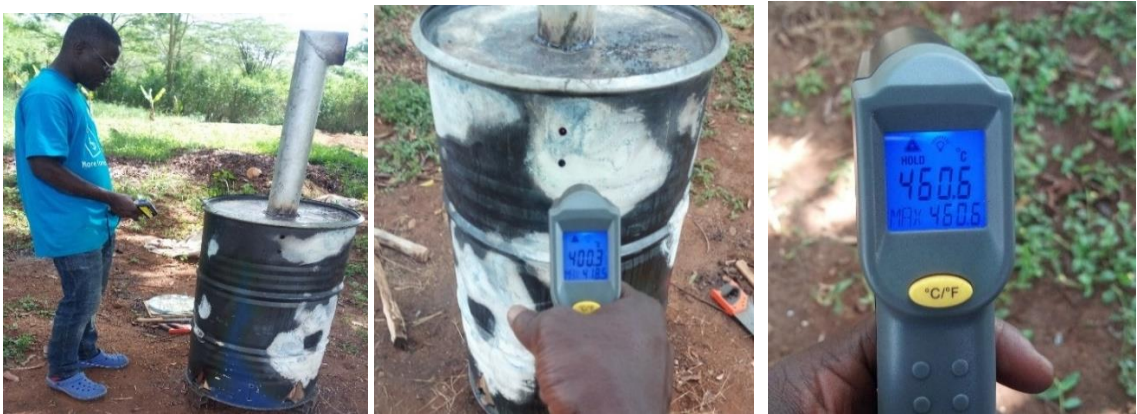
Plate 4: Checking temperature during pyrolysis (Author, 3 rd December 2018).
