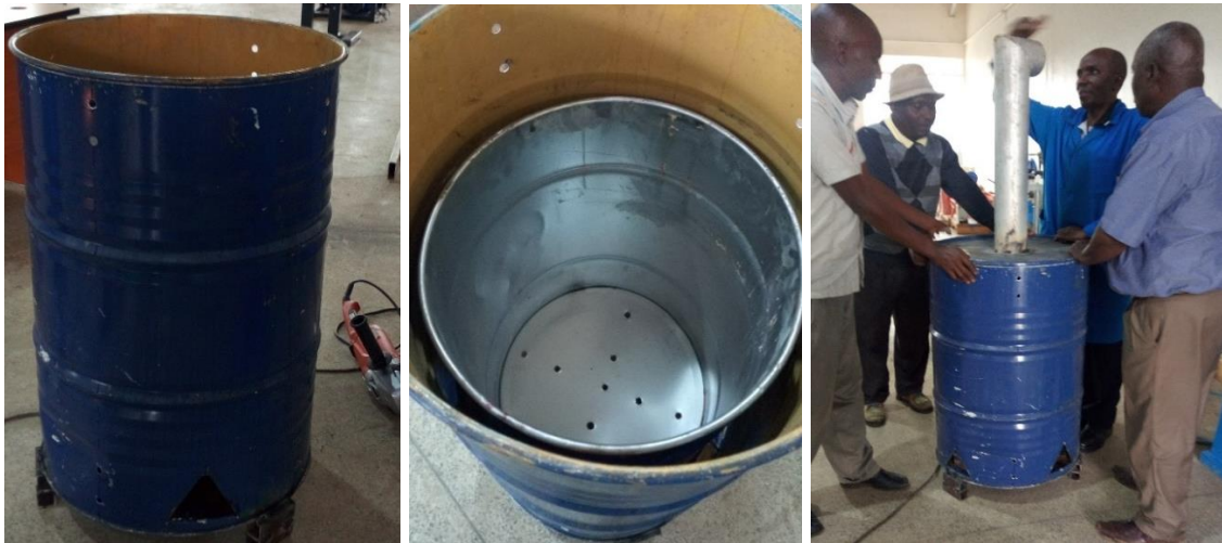
Plate 1: Locally designed oven for biochar production. School of Engineering, Kenyatta University (Author, 19 th November 2018).
