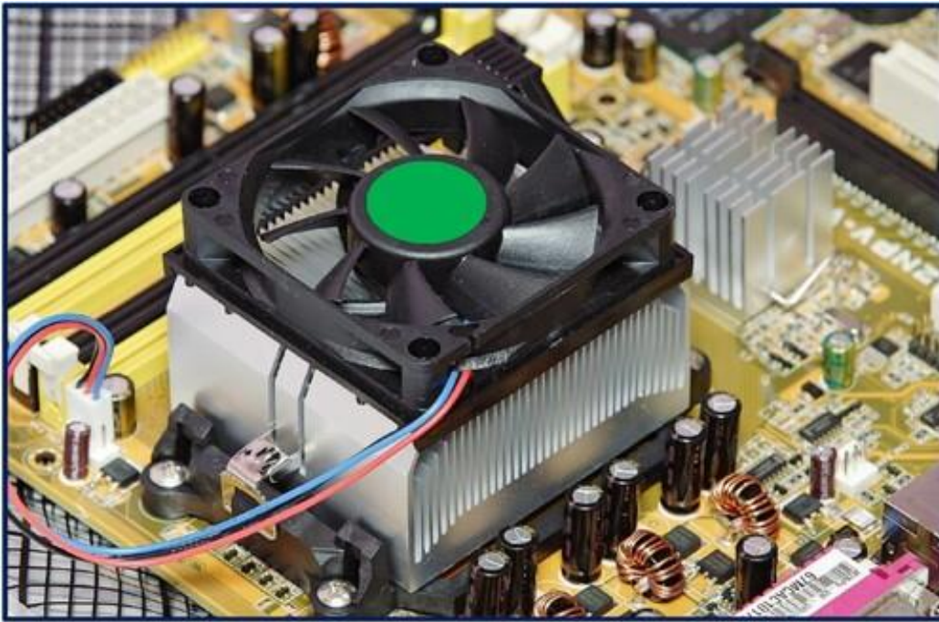
Figure 3.0.1 CPU cooling system model(Venkateswarlu et al., 2024)
