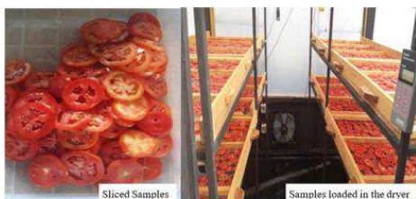
Figure 9. Photo of Sliced and tray loaded with uniformly spread tomatoes in the Solar Greenhouse Dryer.
