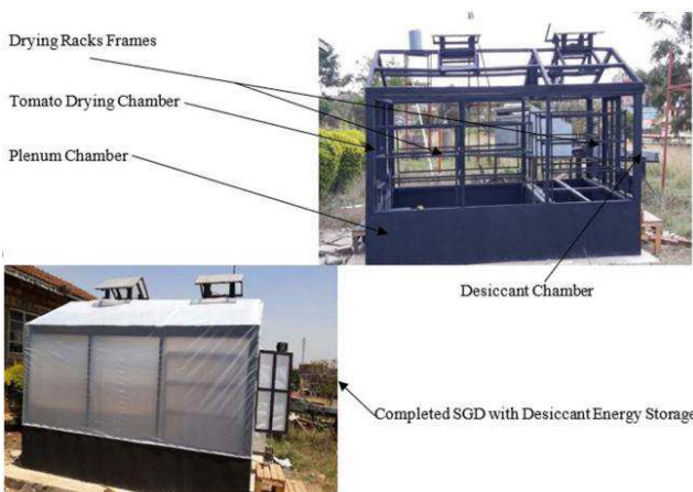
Figure 2. Constructed SGD with Solid CaCl 2 - Clay Desiccant energy storage system Photo.
