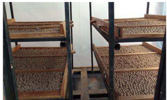
Figure 10. Loaded Solid Clay-CaCl 2 desiccants in the greenhouse desiccant.
