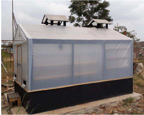
Figure 1. Experimental solar greenhouse dryer incorporated with Solid Clay-CaCl 2 desiccant energy storage system.
