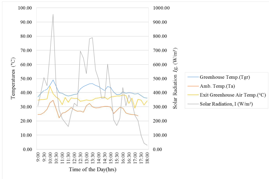
Figure 15. Greenhouse Chamber Typical Temperature and Solar Radiation profile with time During Day 2 on 17th October 2019.
