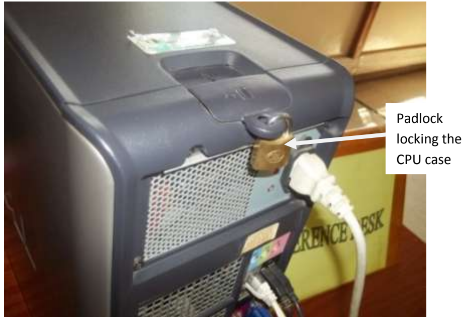
Plate 4.6: A padlock was used to lock the CPU cabinet in one of the libraries
