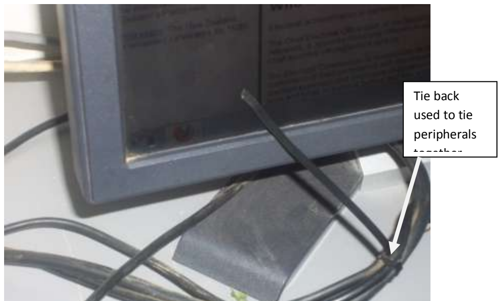
Plate 4.5: Tiebacks/clips used to tie peripherals together in yet another library. Source: Observation.
