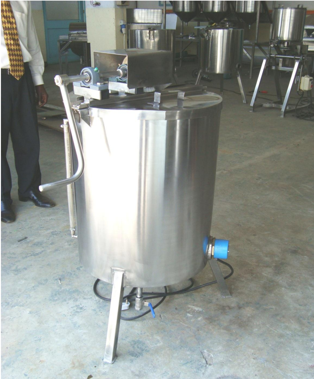
Figure 5. 15: The complete designed and constructed honey extractor-warmer machine
