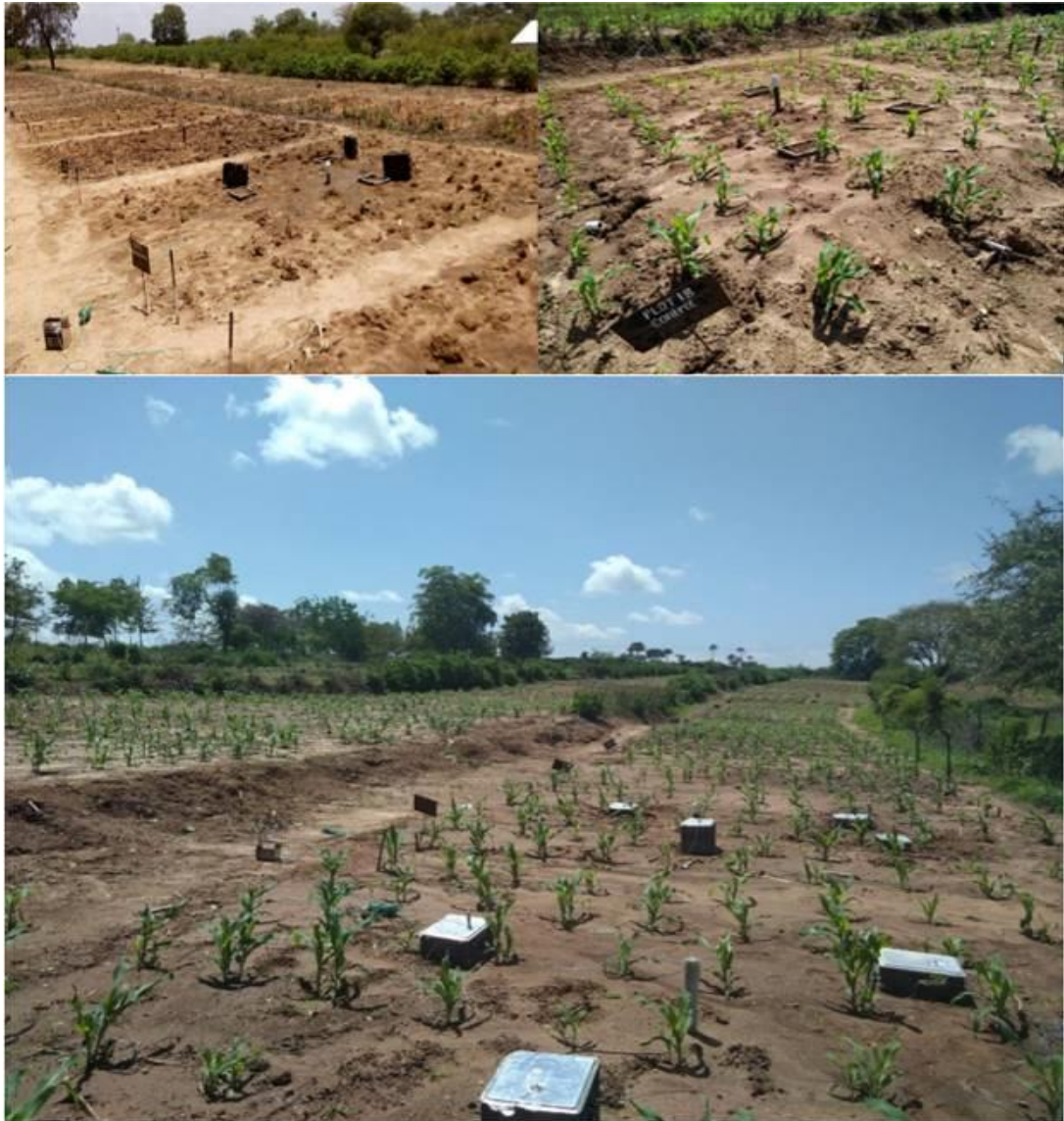
Plate 3.1: Experimental field set with chamber bases installed (Source: Author, 2017)
