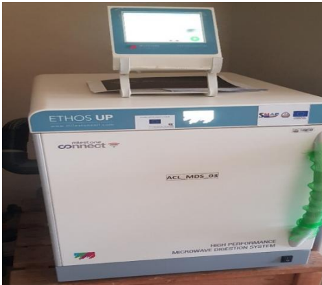
Plate 1 A photo of high-performance microwave digestion systems at KEPHIS Laboratory in Karen, Kenya
