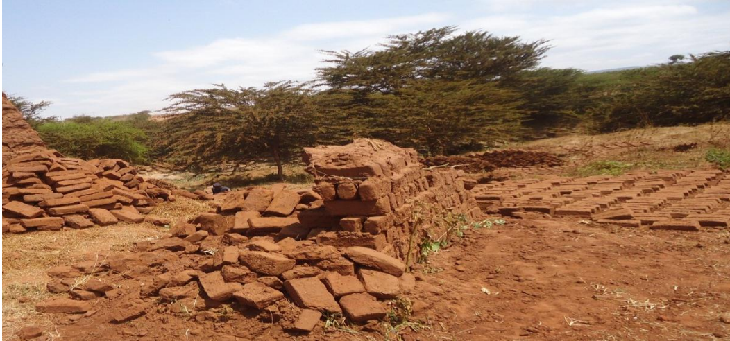
Fig A5: Rough Bricks made from red soil at Emali town for building and construction in Makueni County.
