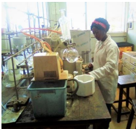
Picture 3: Concentrating Plant Extracts using a Rotary Evaporator (Chemistry Lab, Kenyatta University)
