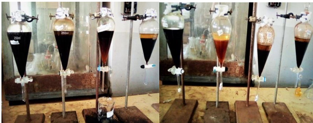
Figure 4: Solvent-Solvent partitioning of plant extracts using Hexane, Dichloromethane, Ethyl acetate, and Methanol (Chemistry lab, Kenyatta University)
