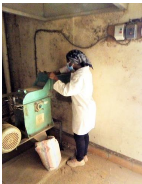
Picture 1: Grinding Plant Samples using a Grinding Mill Machine (Kenyatta University)
