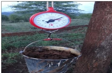
Plate 3.5: Measurement of sediment
