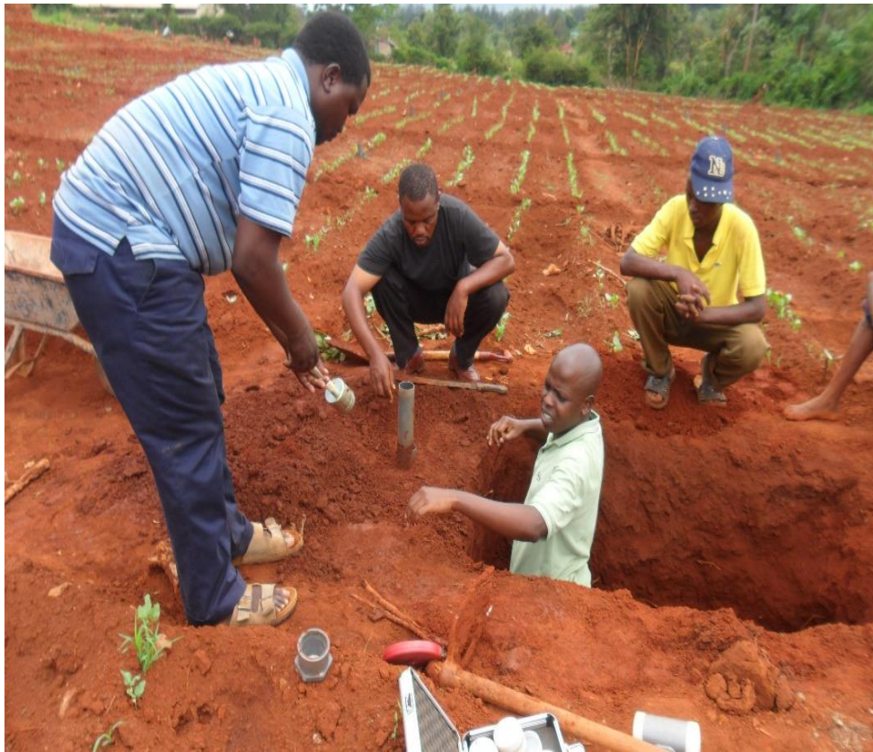
Plate 4: Soil sampling process for bulk density measurement in a profile pit for Diviner 2000 calibration
