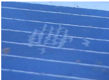
Figure 5.13: Picture of the 10W polycrystalline module defect
