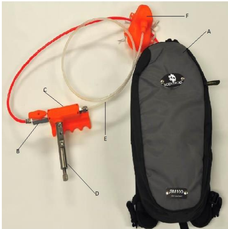
SM 100 overview, A; Air supply backpack, B; Shut off valve, C; Ergonomic handle with Educator underneath, D; Dilution regulator valve, E; Face mask
