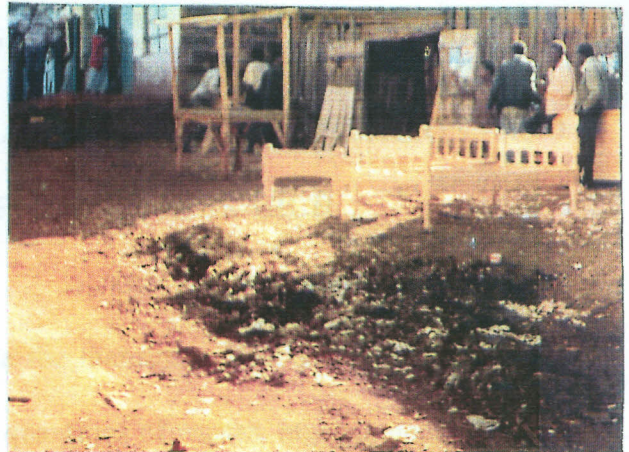
Plate X: Wastes from a workshop strewn near the road. These wastes are always washed away by storm waters where they end up clogging drains and sewers.
