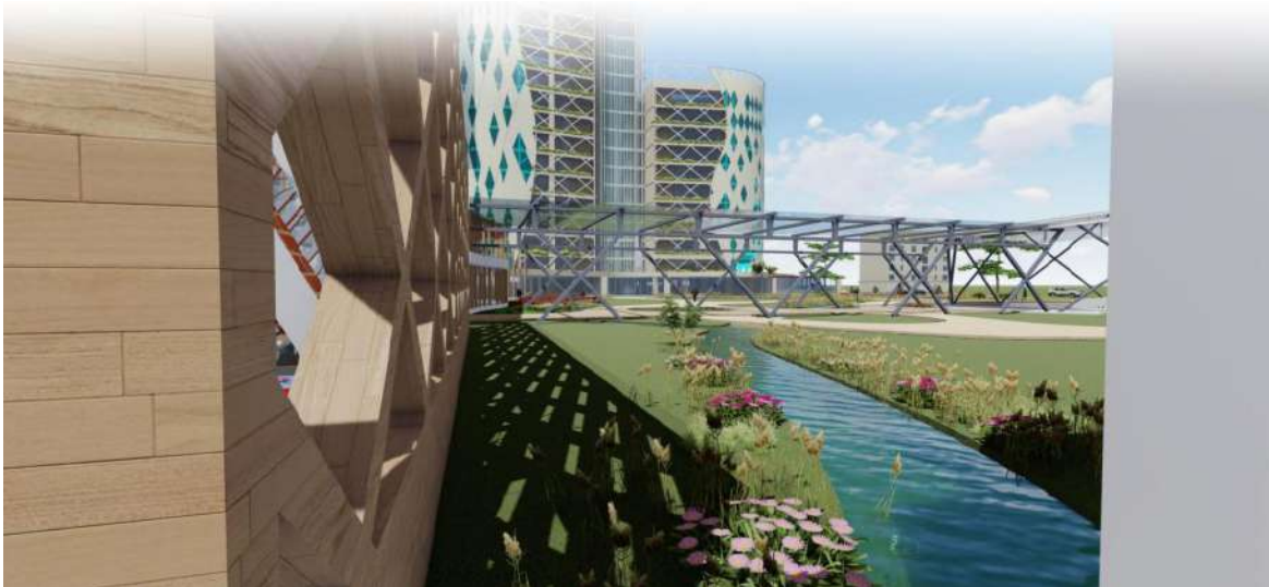
Figure 15: Achieving evaporative cooling by use of artificial rivers. Source: Author generated; 2024.
