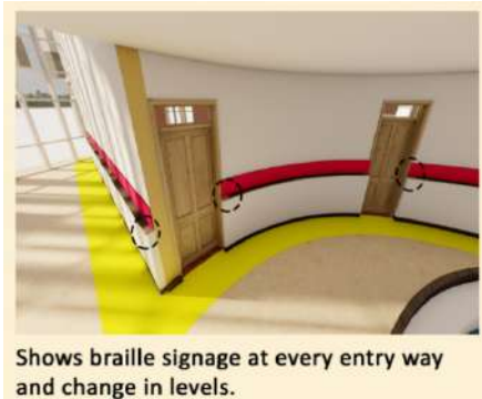
Figure 10: Shows the placement of braille signage along sensory trail wall. Source: Author, 2024.
