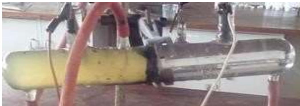
Figure 3.5: The assembled electrochemical cell in this study
