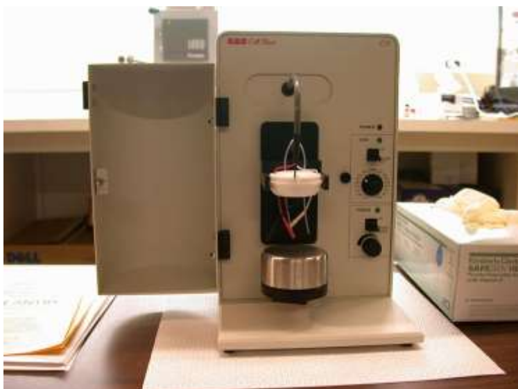
Figure 3.4: Epsilon electro analyzer equipped with a door used in the voltammetry analysis in this work
