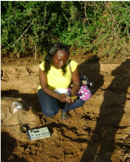
Figure A3 (d): Equipment used in the field. The Geiger Muller counter was used for in situ measurements of radioactivity levels while the GPS was used to locate the sample collection site (Taken on 30/11/2014).
