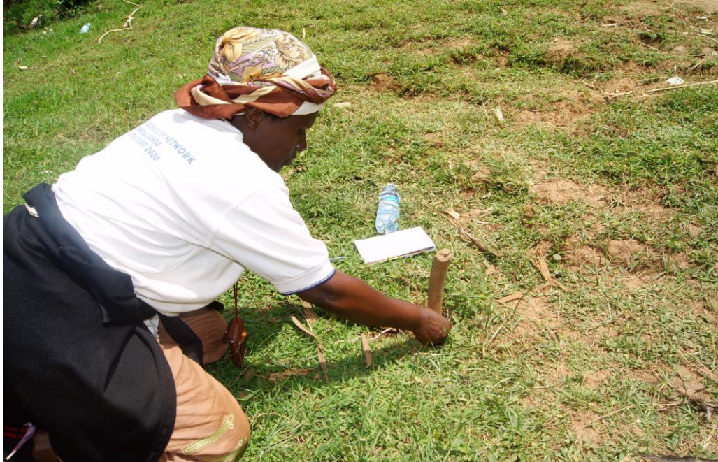
Plate 3.5: Peg displacement measurement to detect likelihood of slope failure (Bukhalasi – Bududa, March 2009)
