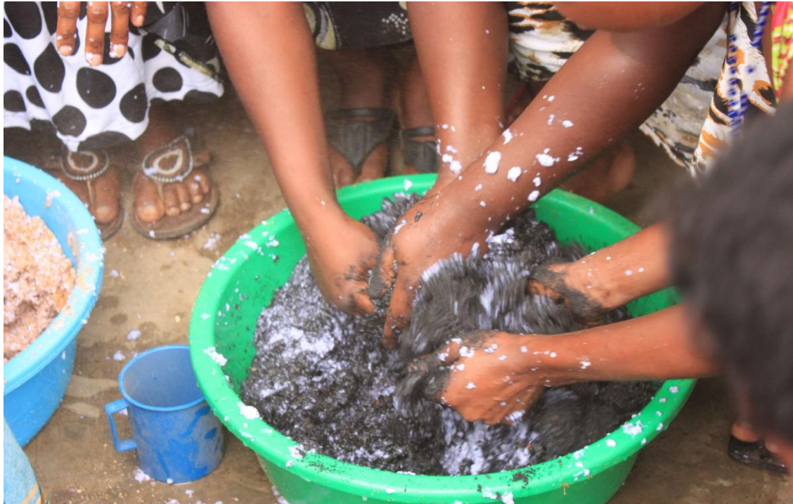
Plate 5. 1: Mixing of sawdust and charcoal dust (Source: Maa-Briquettes Narok)
