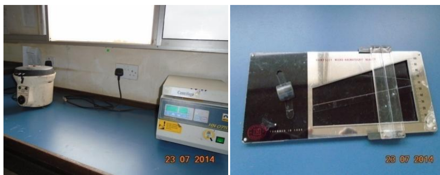
Figure 28: Equipment for determination of packed cell volume (PCV)
